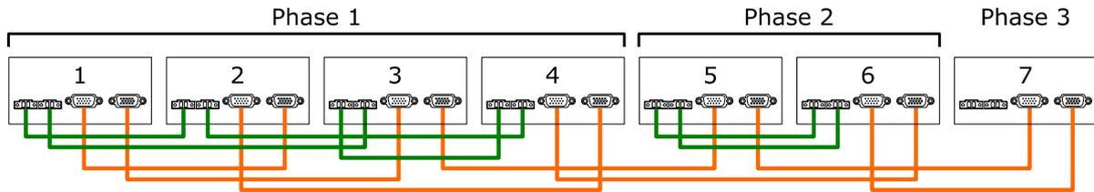
Figure 42: Communication wiring of seven inverters in a 3-phase system (4 + 2 + 1)
