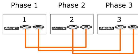
Figure 27: Communication wiring of three inverters in a 3-phase system
