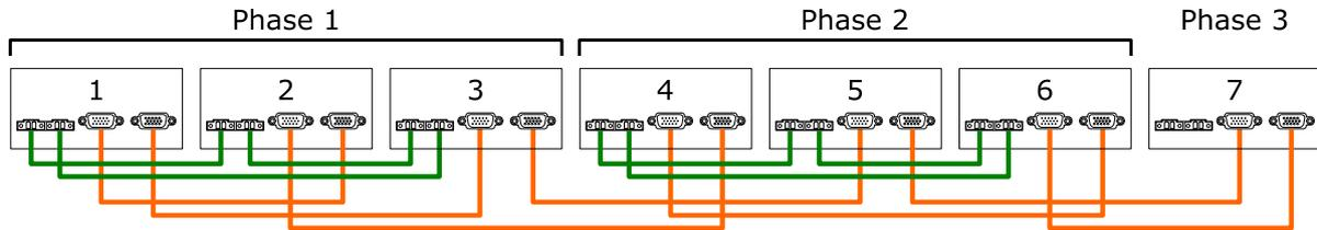
Figure 41: Communication wiring of seven inverters in a 3-phase system (3 + 3 + 1)
