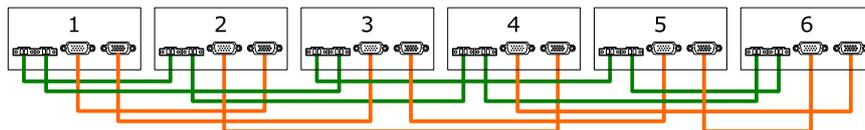
Figure 22: Communication wiring of six parallel inverters on single phase
