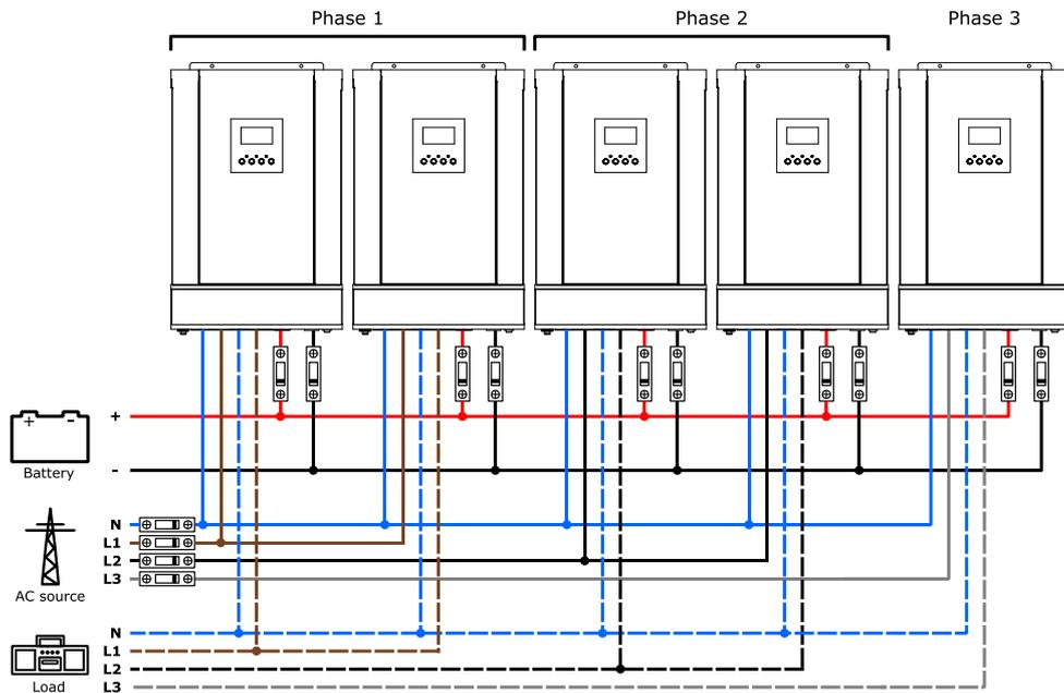
Figure 32: Wiring of five inverters in a 3-phase system (2 + 2 + 1)
