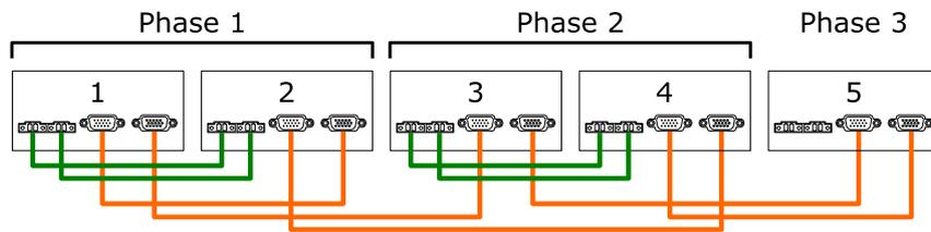
Figure 33: Communication wiring of five inverters in a 3-phase system (2 + 2 + 1)
