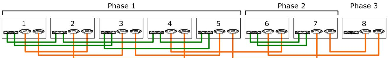
Figure 46: Communication wiring of eight inverters in a 3-phase system (5 + 2 + 1)
