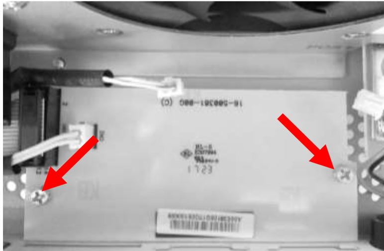
Figure 4: Remove screws on beige board
