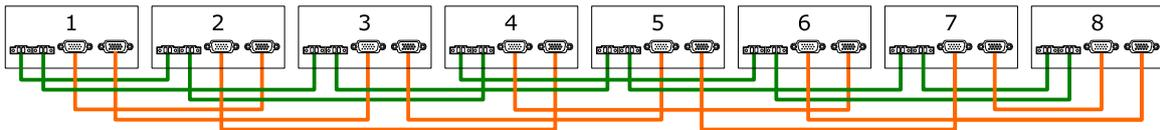
*Figure 24: Communication wiring of eight parallel inverters on single phase*
