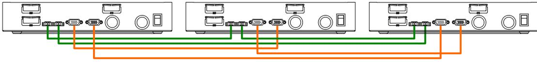
Figure 17: Communication wiring of three parallel inverters on single phase
