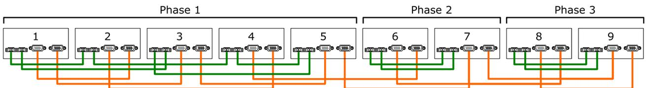
Figure 53: Communication wiring of nine inverters in a 3-phase system (5 + 2 + 2)
