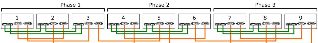
Figure 50: Communication wiring of nine inverters in a 3-phase system (3 + 3 + 3)
