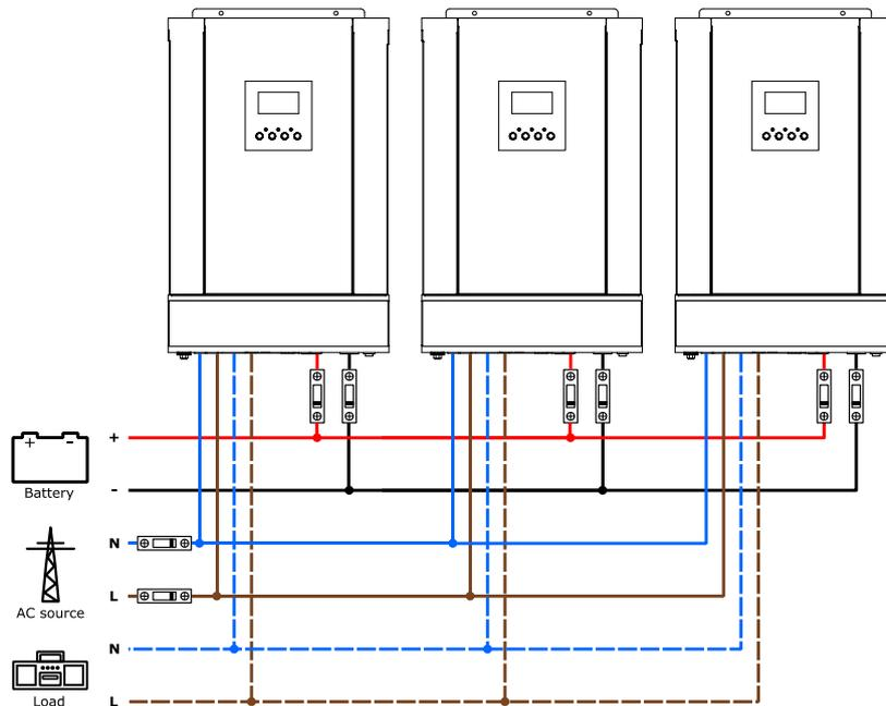
Figure 16: Wiring of three parallel inverters on single phase
