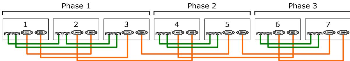
Figure 43: Communication wiring of seven inverters in a 3-phase system (3 + 2 + 2)
