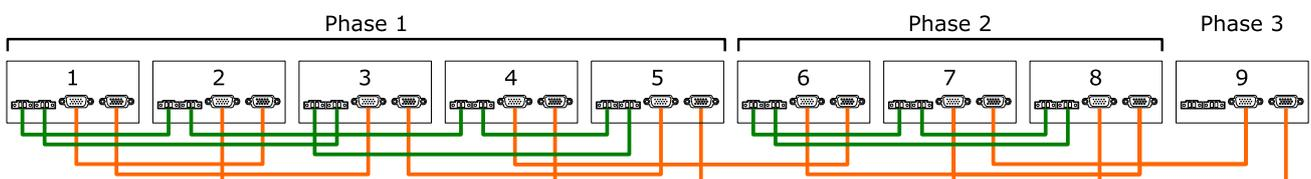
Figure 54: Communication wiring of nine inverters in a 3-phase system (5 + 3 + 1)
