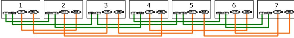
*Figure 23: Communication wiring of seven parallel inverters on single phase*
