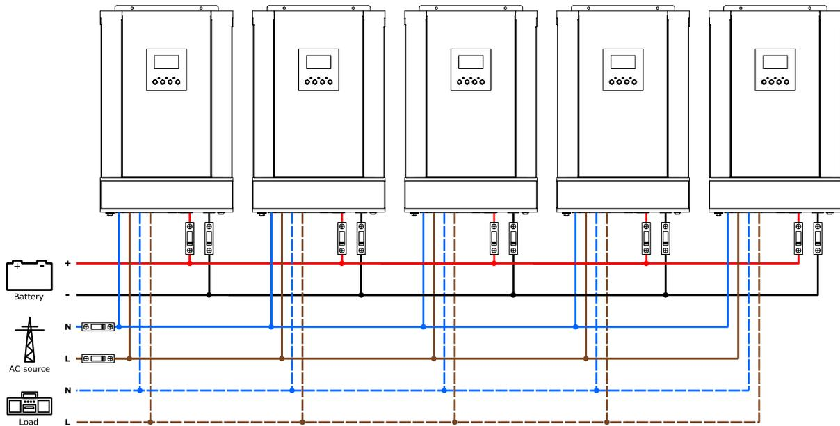
Figure 20: Wiring of five parallel inverters on single phase
